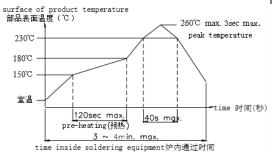
Automatic Flow Soldering (自动焊接) Caution: the condition mentioned above is a temperature on the PWB surface on which parts are mounted. There are cases where PWB temperature greatly differs from switch's surface temperature depending on PWB material, size, thickness, etc. The switch's surface temperature shall not allowed to exceed 260℃
