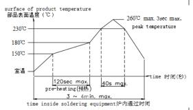
Automatic Flow Soldering (自动焊接)
