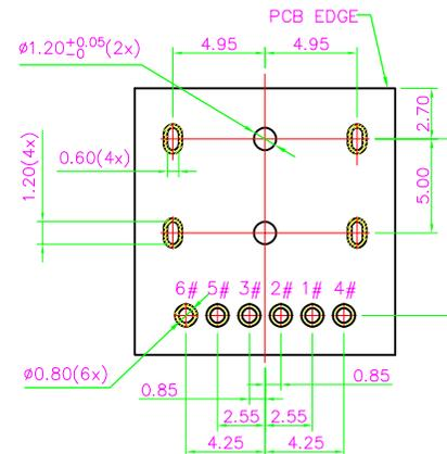
PCB HOLES(TOP VIEW) t=1.2mm
